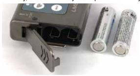
Spring contacts inside the compartment and nickel plated contacts on the door keep the batteries from rattling and provide reliable electrical contacts. The unit is protected from reverse battery polarity electrically, and by the insulated contact plate in the battery door.
